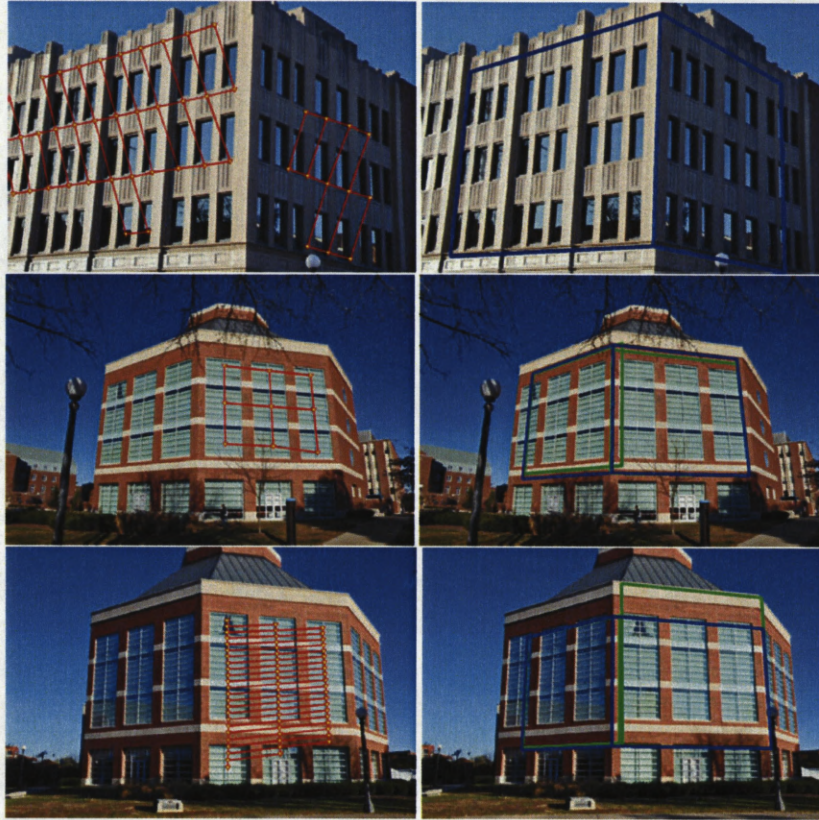
Figure 12: Comparison the lattice detection [19] (left) against our compression based segmentation (right). In the right images, green shows the segmentation result and blue is the refined solution after intersection detection.
