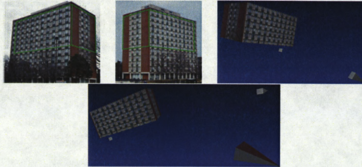
Figure 1: Left Pair: Example of matched facades of a building. Right Pair: Automatically reconstructed 3D model from only four uncalibrated images around the building by our method. Each image covers a pair of facades. The pyramids show the estimated location of cameras.
