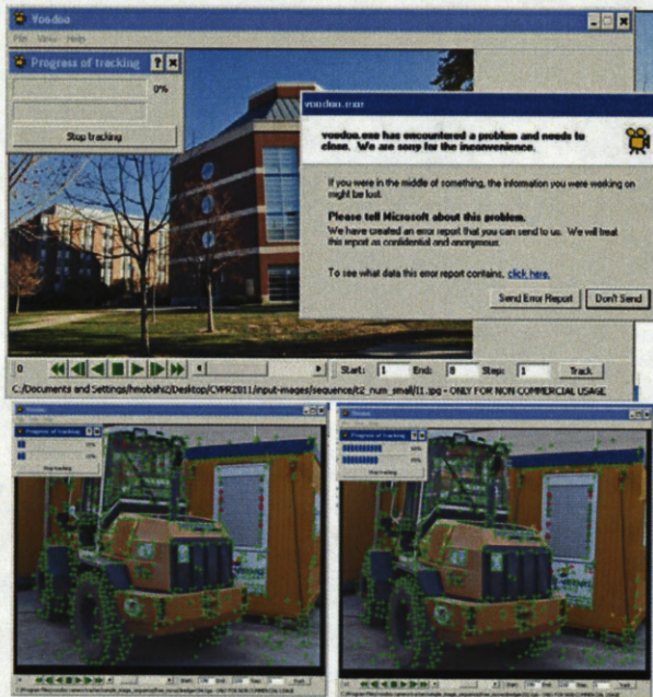
Figure 14: Voodoo camera tracker crashes on our data (top), while it works on the example sequence that comes with a package (bottom). The latter sequence is almost a video sequence, where most of the local features in each frame can be reliably tracked in the next frame. This is obviously not the case for our data where the two successive images are significantly different by any local measure.
