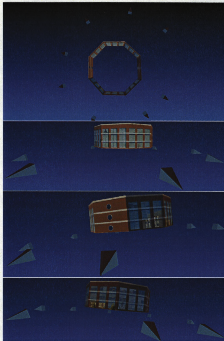
Figure 11: Top and frontal views of the recovered building. Each pyramid shows the estimated location of a camera.
