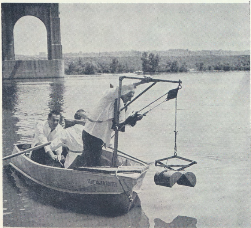
Bottom-sampling device is lowered into river to collect samples for research on improving water quality
