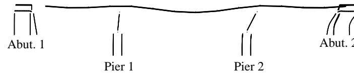
(d) Deformed bridge shape at the state with a 100-mm deck center displacement (deformation is magnified by 40 times)
