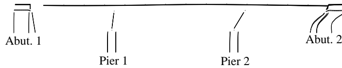
(c) The predominant mode shape (Mode 1) in the longitudinal direction at the state with a 100-mm deck center displacement
