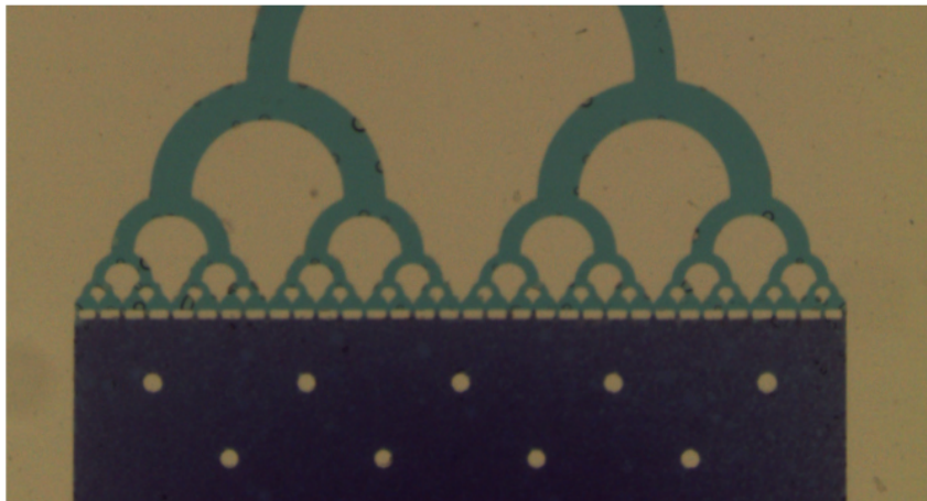
Figure 5.3: Zoomed-in schematic of the bead capture region. The bottom picture is an actual picture of the device colored with dye. This shows the distribution of the solution over the entire bed of resin, with the support posts clearly visible.
