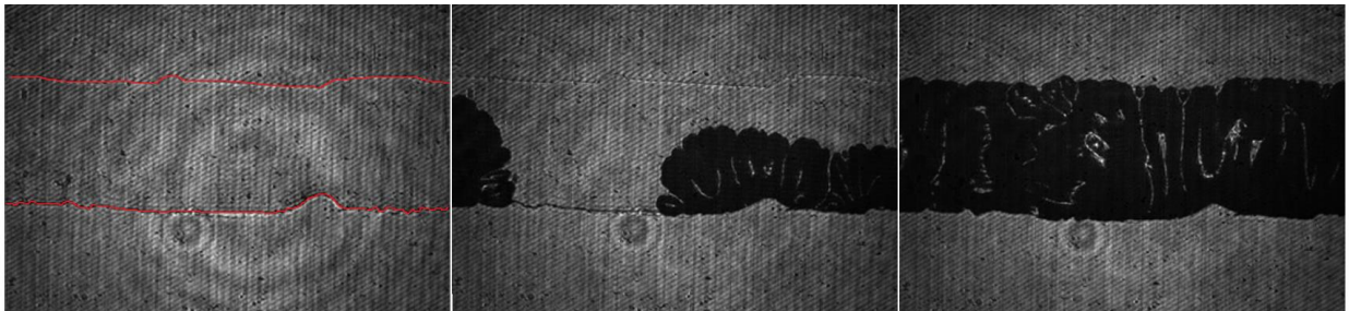
Fig. 22: Time lapse from left to right of a Pd ridge (outlined in red) exposed to 4% hydrogen in nitrogen showing buckling, delamination, and plastic deformation.
