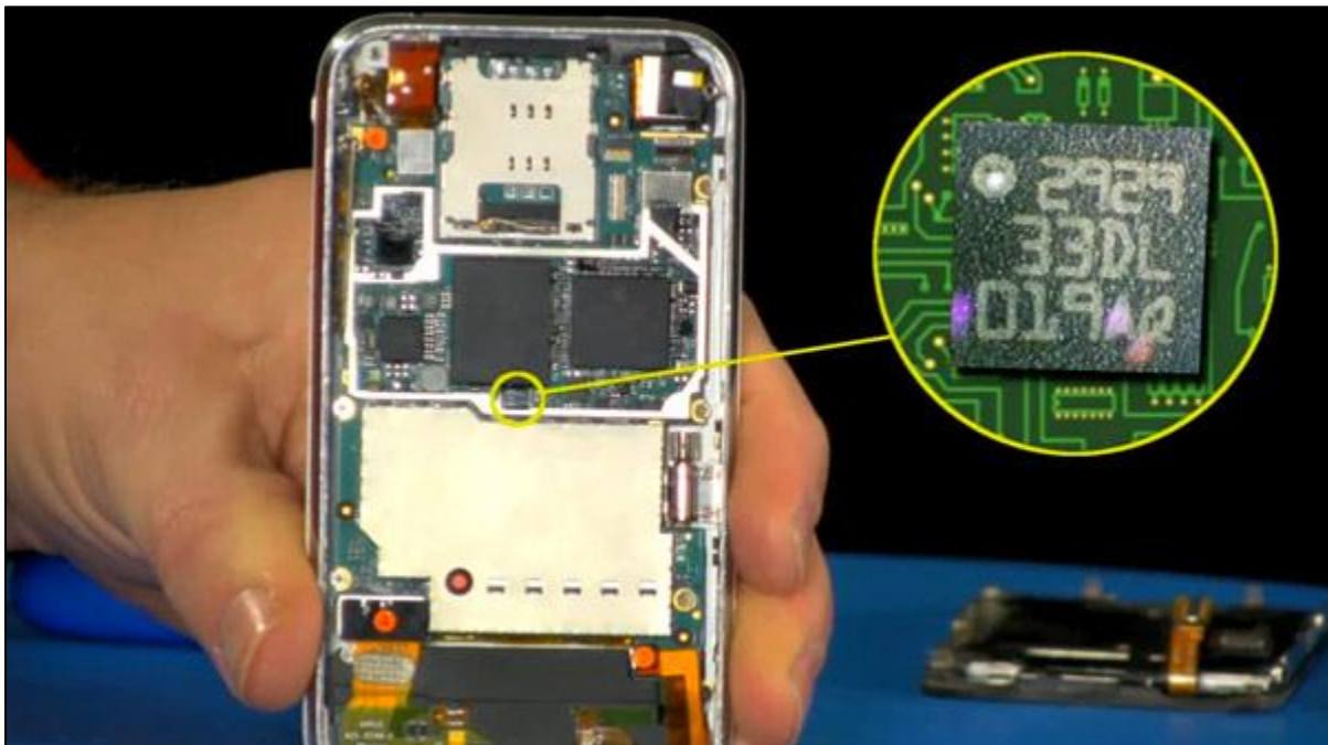
Figure 5.2: A Typical Accelerometer Used in Smartphone [82]
