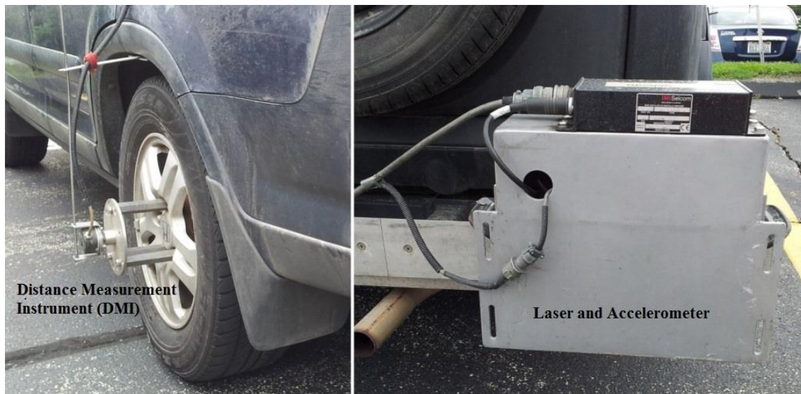
Figure 4.9: Automated Pavement Profiler and Equipment on a Typical Data Collection Van
