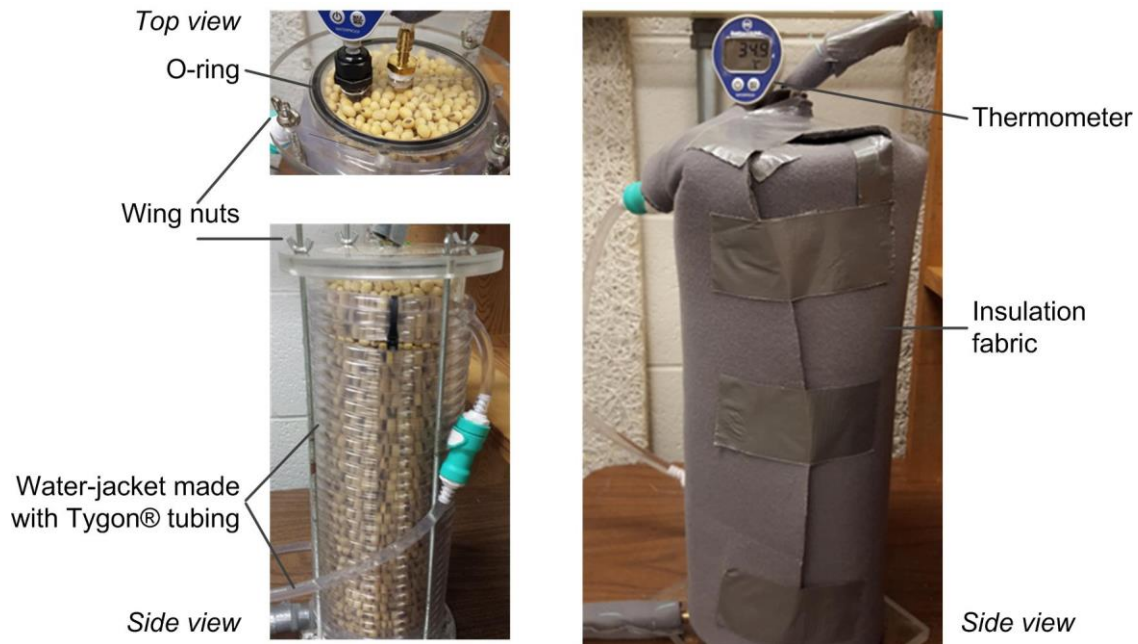
Figure C.2. Soybean-filled grain column before and after being wrapped with insulation.
