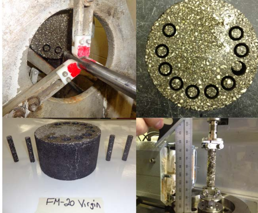
Figure J.2 Specimen preparation process for FAM specimens including cutting, coring, and test setup.
