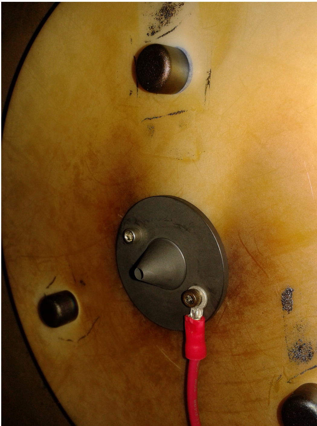
Figure 4.7: The short skimmer on the Teflon mount in the source chamber.
