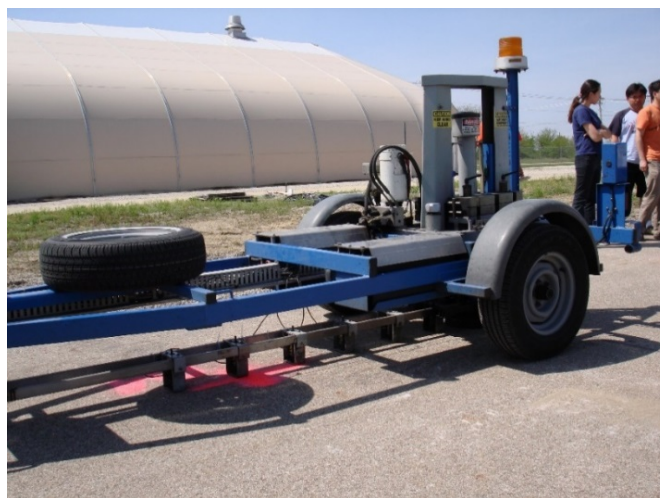
Figure 2.1: Photo of the Dynatest falling weight deflectometer device at the University of Illinois.
