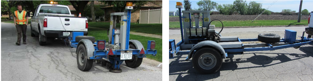
Figure 3.1: Conducting FWD tests in selected local road pavement sections in Illinois.
