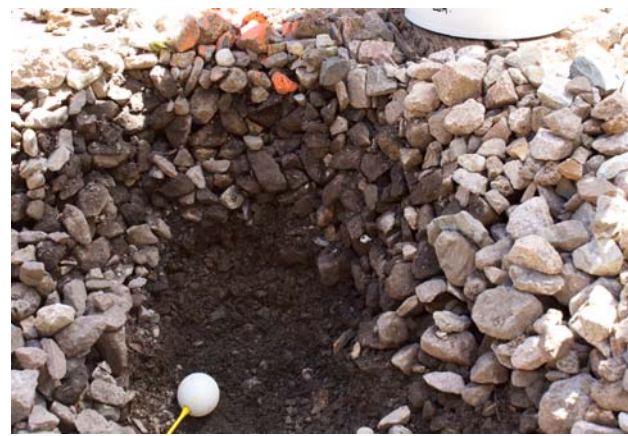
Figure 7.14(b) Aggregate Sampling Track Location along a Mainline Freight Railroad in Mississippi (2 in. White Calibration Ball)
