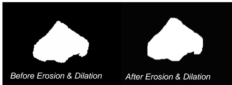
Figure 2.13 Smoothing the Surface of a Particle Image Linking to Surface Texture Before and After Cycles of Erosion and Dilation [46]
