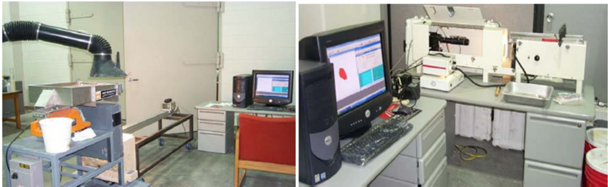
Figure 2.4 Buffalo Wire Works (PSSDA) System for Evaluating Size/Form for Coarse (Left-Side Picture) and Fine (Right-Side Picture) Aggregates [38]
