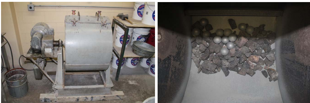
Figure 4.2 LA-Abrasion Testing Apparatus and Sample with Steel Balls
