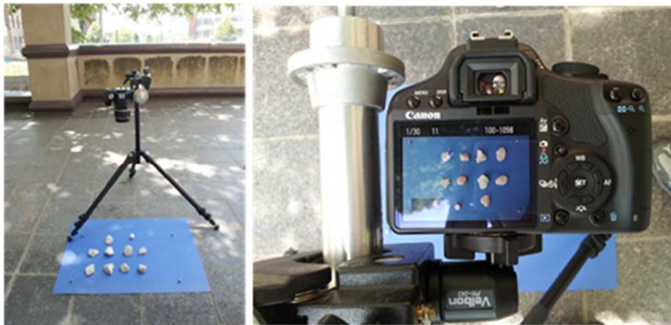
Figure 7.13 Camera Setup for Aggregate Imaging with Blue Background in an Outdoor Setting (Left: Front View of Camera and Tripod, Right: Top View Camera Screen)
