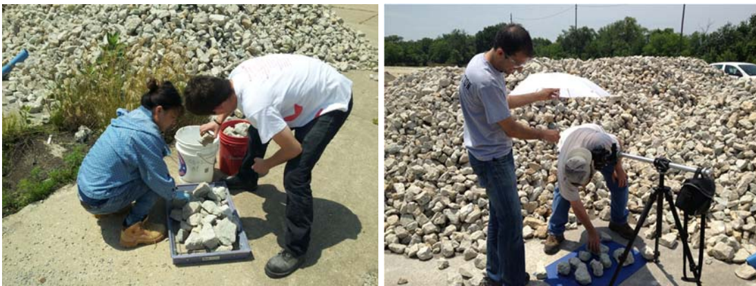
Figure 7.15 Left: Separating Large Particles with Sizes above 3 in. (76 mm) Right: Image Acquisition in the Field with DSLR Camera and Blue Background
