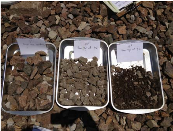
Figure 7.14(a) Aggregate Collected at the Surface or 0 in. (Left), 8 in. (Middle), and 16 in. (Right) Ballast Depths
