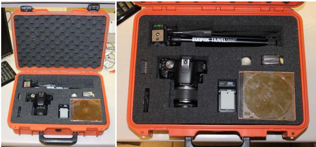
Figure 7.12 Aggregate Imaging Kit Including DSLR Camera, Accessories, Tripod and Image Calibration Tools
