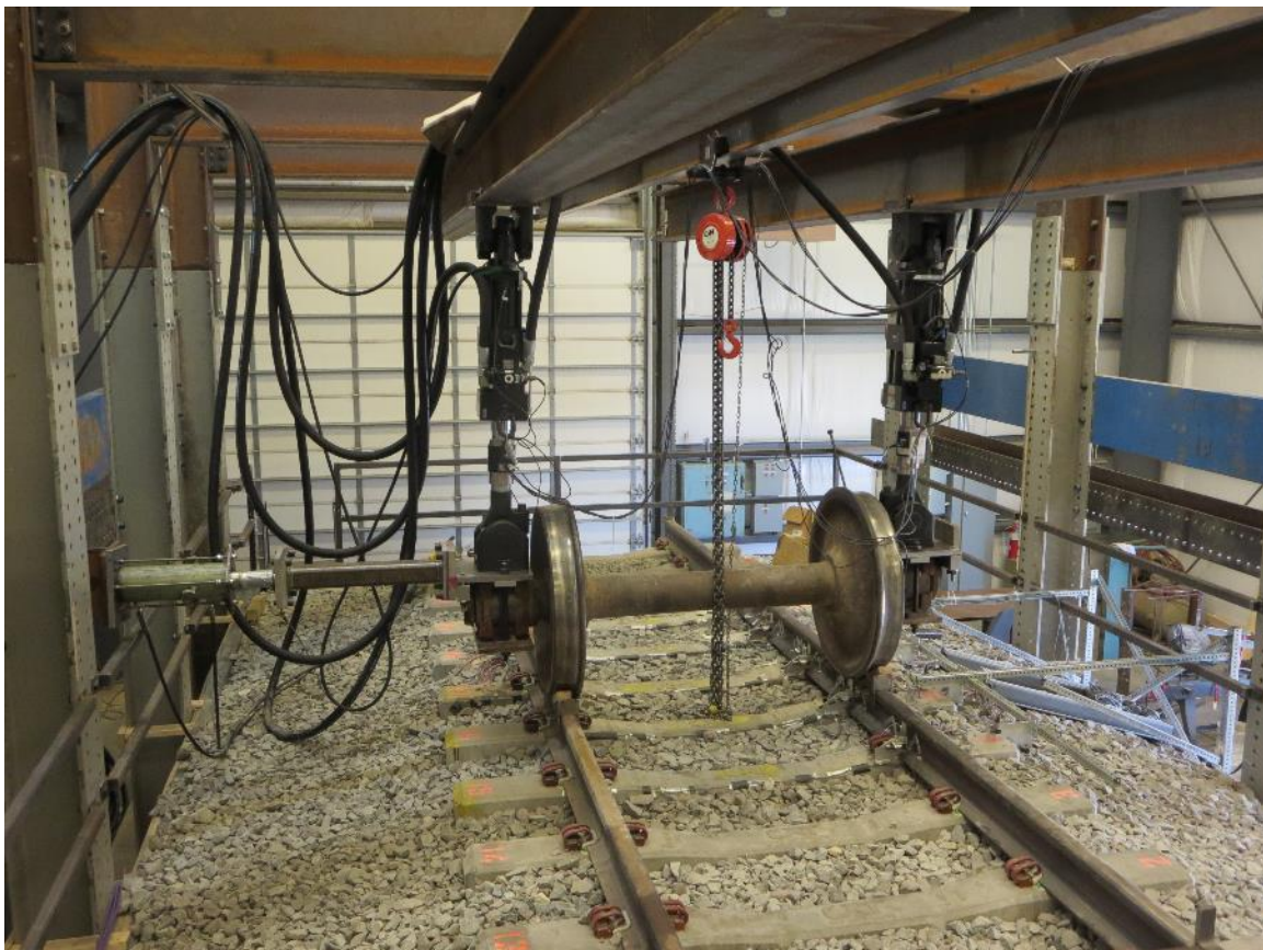
Figure 2.2 Track loading system (TLS) installation during experimentation
