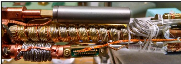
Figure 5.1: dc-SQUID sensor in a Nb-enclosure mounted on the 1K plate of the Oxford He-3 system.
