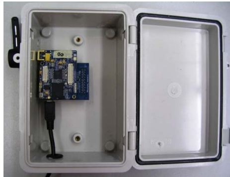
Figure 8.5. Enclosure configuration: gateway Node.
