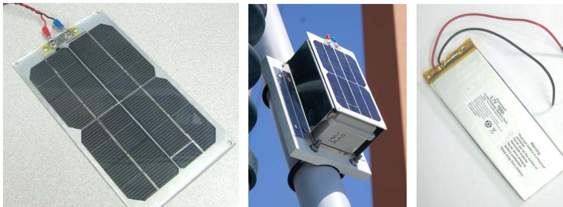
(a) SPE-350-6 (9V-350mA, Solarworld) (b) on cable node (c) Rechargeable battery Figure 6.7. Solar panel and rechargeable battery for Jindo Bridge SHM.
