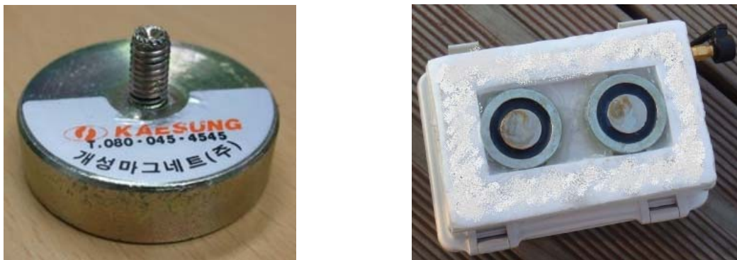
(a) 10 kg capacity one-directional magnet (b) Bottom of the leaf nodes
