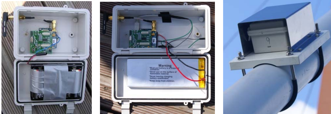
(a) Battery-powered node (b) Solar-powered node (c) Cable node
