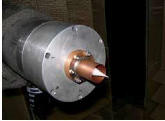
Figure 3.26: Center body installed in facility.
