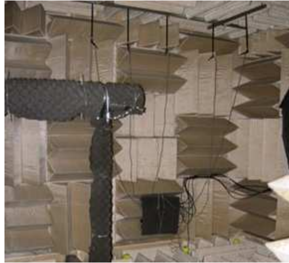
(b) In-chamber microphone positioning.
