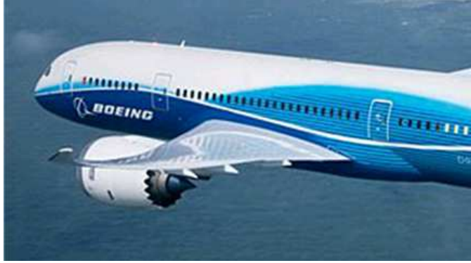
Figure 3.1: Boeing 787 “Dreamliner” showing the use of chevrons for noise mitigation in practice. Photo from www.boeing.com .
