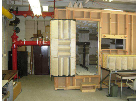
Figure 2.1: The anechoic jet noise facility.
