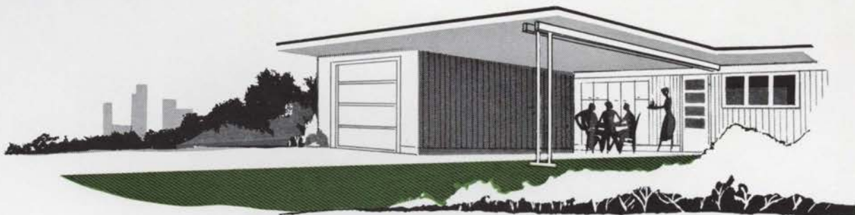
Instead of a double garage, this house has a carport and a single garage. The carport also serves as a covered outdoor living area. Storage space is provided in one wall of the carport.
