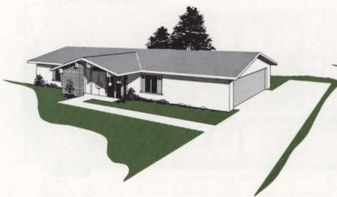
A garage facing the side lot line requires more side yard, but the door is not as dominant in the appearance of the house.
