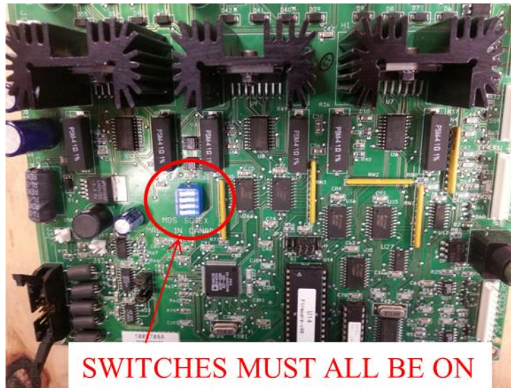
Figure A.6: oMALDI control/power board with configuration switch labeled.
