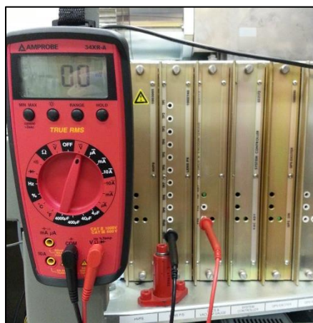
Figure A.3: Proper configuration of a digital multimeter for QSTAR quad chamber pressure measurement.
