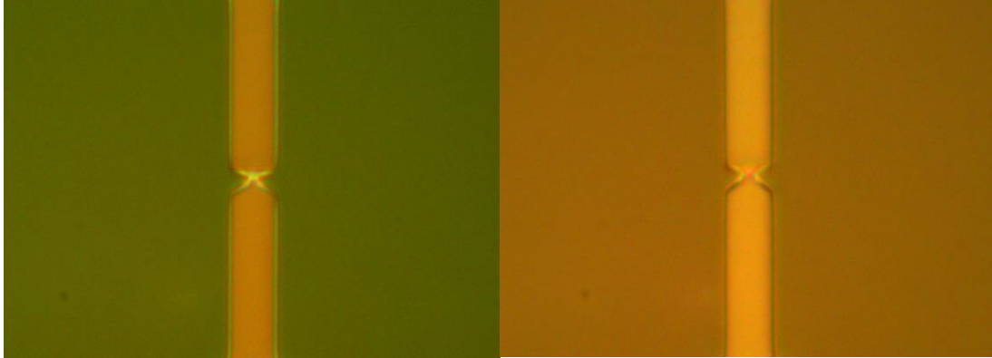
Figure 4.12: Oxygen plasma clean destroys Dolan bridge made of PMMA. Left before oxygen plasma clean. Right: After oxygen plasma clean.
