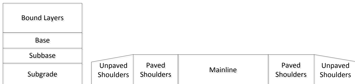
Figure 3.1 Pavement components and structure considered.
