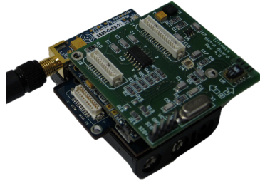
Figure 3.2: Imote2 fitted with SHM-A sensor board and external antenna.
