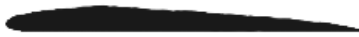
Figure 4.11: A sketch representative of the thin airfoil used on the two balsa gliders.
