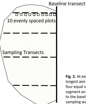
**Fig. 2.** At each site, a baseline transect was placed on the longest axis of the wetland. This transect was divided into four equal segments. At a random point within each segment an additional transect was placed perpendicular to the baseline, creating four transects along which sampling was conducted
