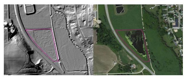
**Fig. 4.** Mitigation site in Stephenson County Illinois, outlined in pink. Left: digital terrain model (DTM) derived from LiDAR data used in calculating floodwater storage potential. Right: Orthographic image of study area.
