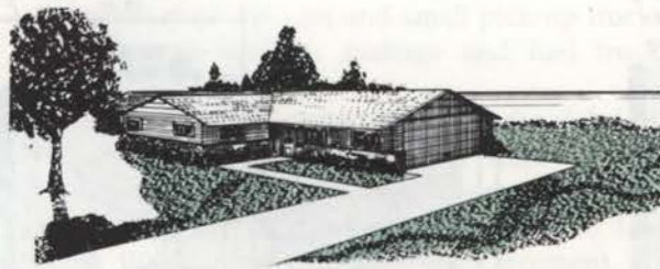
A garage facing the side lot line requires more side yard, but the door is not as dominant in the appearance of the house.
