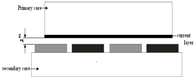
Figure 6: Schematic Representation of Unslotted Primary Core (from Ref. [2]).
