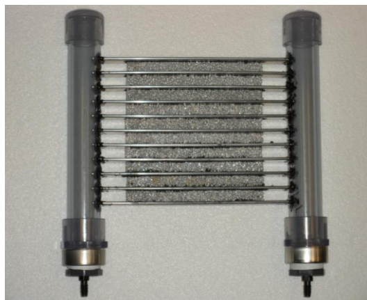
Figure 2.3 Flat tube metal foam heat exchanger (10 PPI metal foams)
