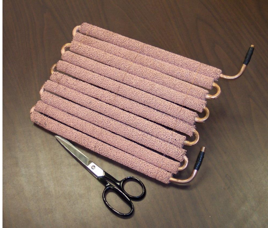
Figure A.2 Metal foam heat exchanger-Round copper tube annular configuration
