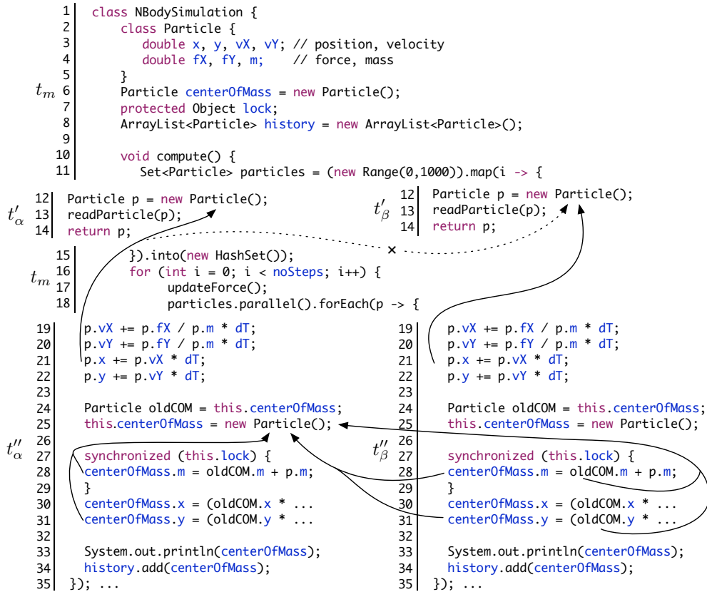
Figure 2.1: Visual representation of how our analysis sees a simple N-body simulation implementation. Each block of code is labeled with the abstract thread that executes it, e.g., t'_\alpha . The arrows show points-to relations from variables to allocation sites, e.g., variable p at line 21 in thread t'_\alpha may point to the abstract object instantiated on line 12 in thread t'_\alpha . Only relevant points-to relations are shown. The dashed crossed arrow represents an abstract points-to relation that would not appear in any real execution, so it is correctly missing in our model.
