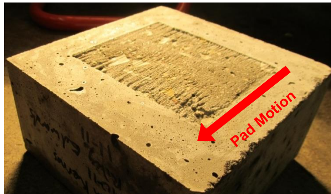
Figure 4.3 Increased abrasion along pad edges of concrete specimen after deterioration test
