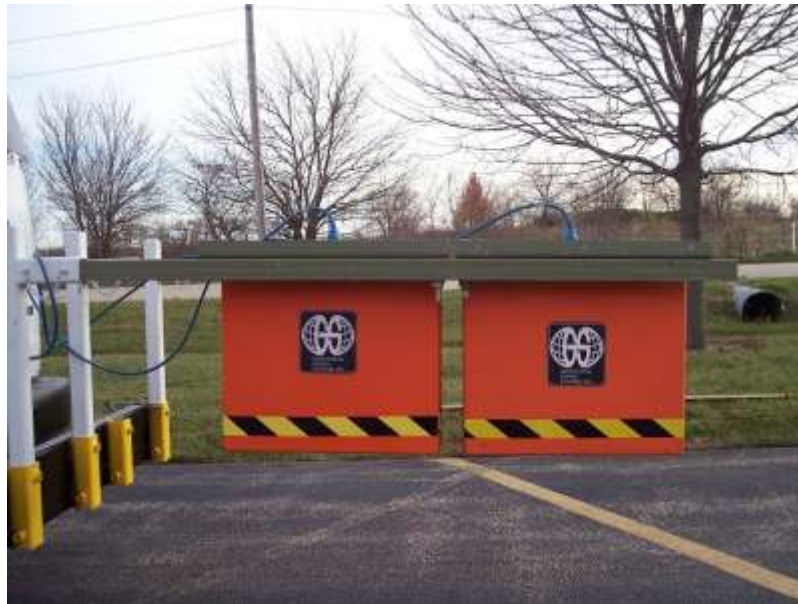
Figure 3.50 GPR antenna systems used for the XCMP method.
