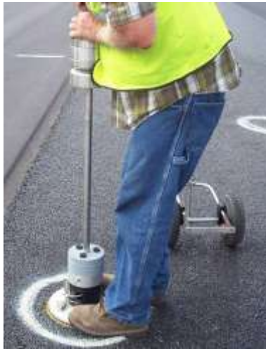
Figure 2.4 Light weight deflectometer.
