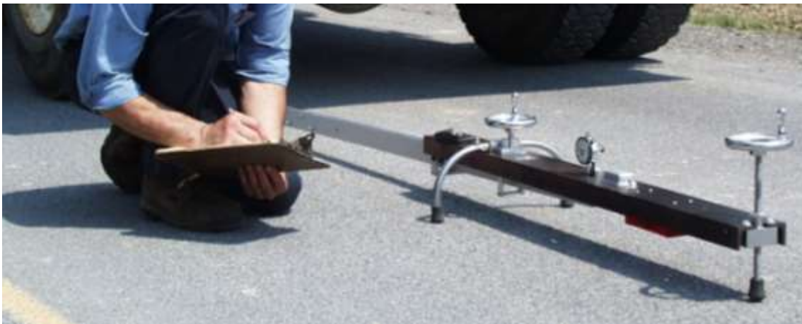
Figure 2.1 Benkelman Beam for pavement deflection measurement.
