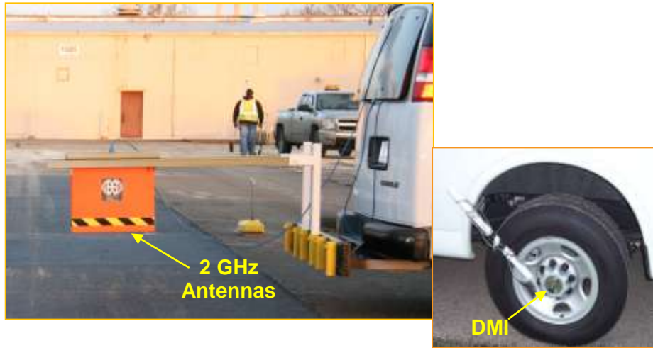
Figure 3.23 2-GHz air-coupled GPR system.
