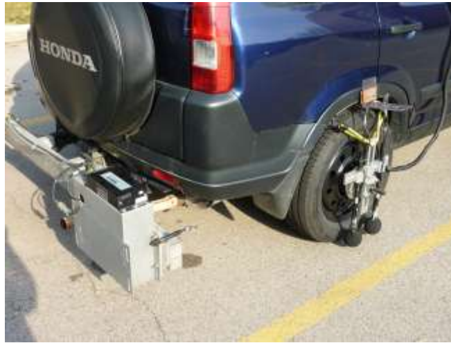
Figure 2.15 Laser device mounted in the back of a van.
