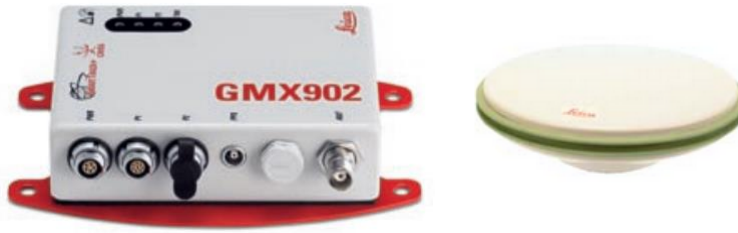
Figure 6.15. Leica GMX902 dual-frequency GPS receiver (left) and AX1202 antenna (right) 0.2mm RMS accuracy, 2.4W power consumption, and up to 20Hz sampling rate (Leica, 2005).
