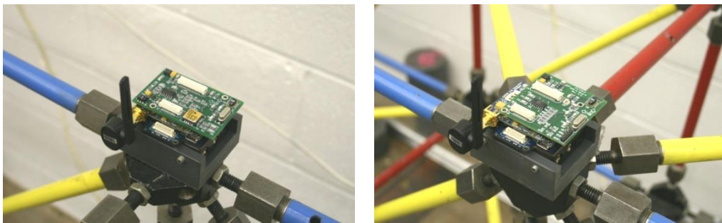
Figure 6.4. Imote2 sensor with SHM-H board (left) and with SHM-A board (right).
