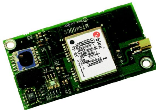
Figure 2.9. MTS420CC (with GPS module) board for Micaz platform (MEMSIC 2011).
