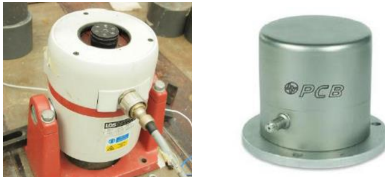
Figure 4.5. Electrodynamic shaker (left) and PCB393C accelerometer (right).
