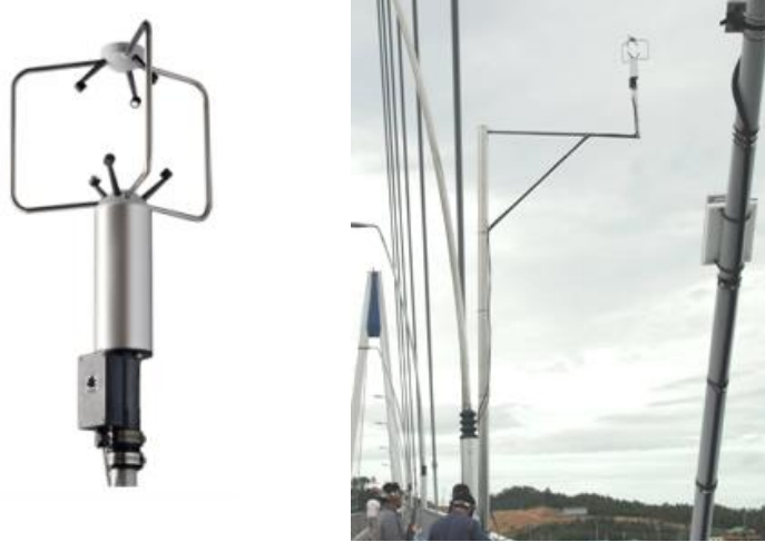
Figure 7.11. RM Young 8100 ultrasonic 3D anemometer (left) and installation on girder (right).
