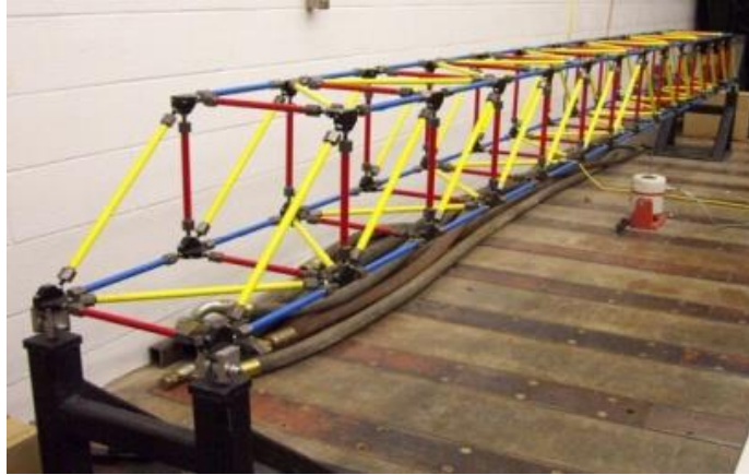
Figure 6.3. Simply supported 16-bay truss structure.
