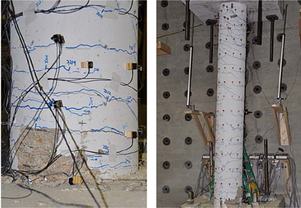
Figure C.8 Pier 1 Cracking Patterns
