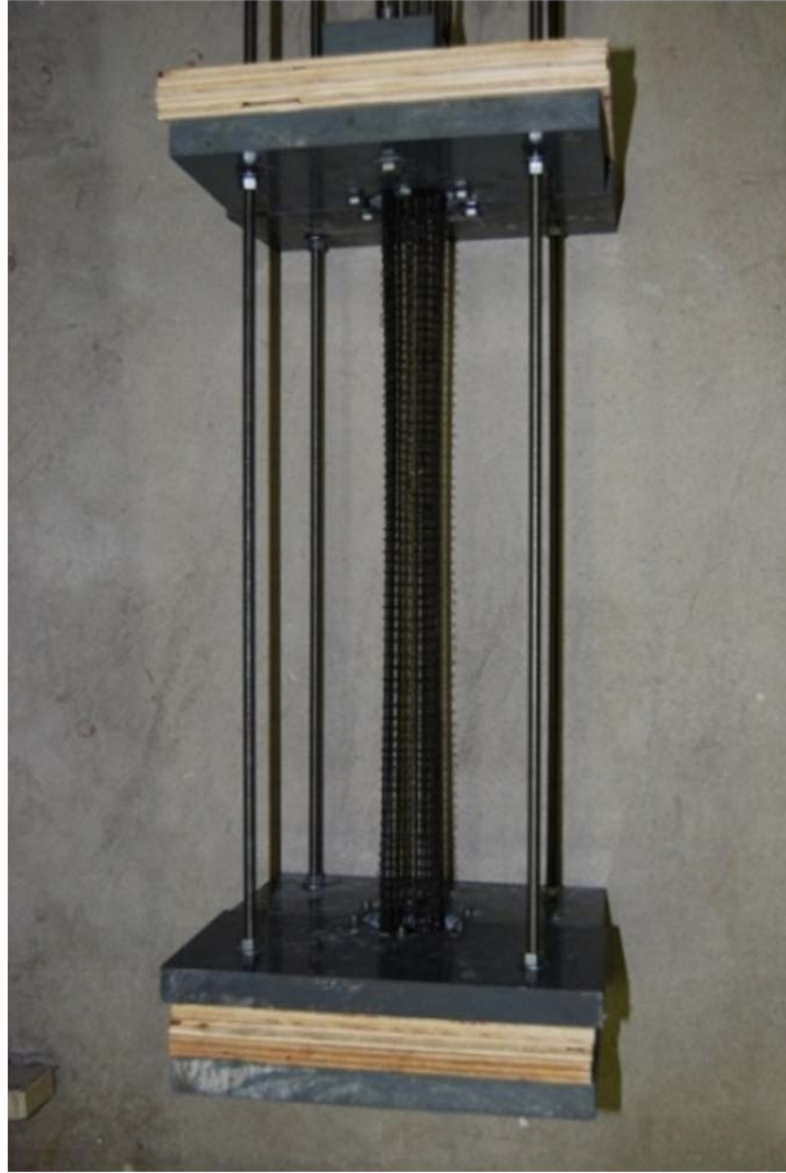
Figure A.9 Small-scale reinforcement cage and cap formwork
