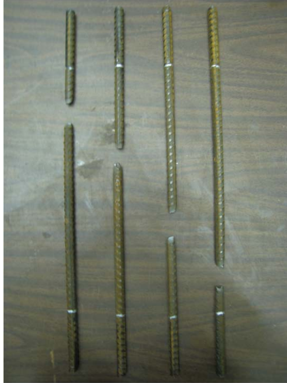
Figure A.11 Necking and rupture of 1:3 scale longitudinal reinforcing bars
