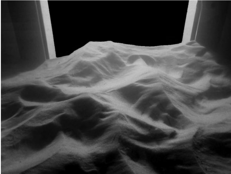
Figure 5.8: Bedform phase state: 3D Symmetric Ripples. Flow Conditions: Oscillatory Condition: U_o = 0.50 \text{ m s}^{-1} and T = 6 \text{ s} . Unidirectional Condition: U_u = 0.00 \text{ m s}^{-1} . The window on the back of the picture is 0.60 m wide.
