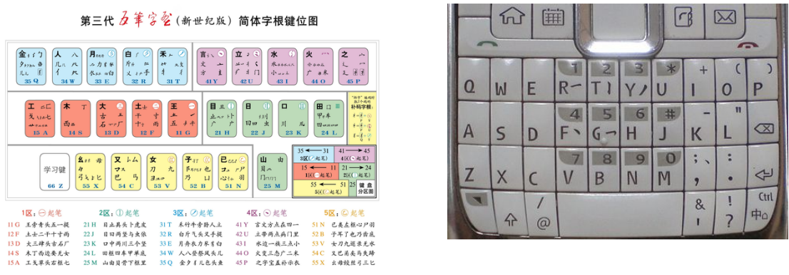
Figure 1. Wubi method input keyboard and cellphone using character stroke system .The five regions are blue, purple, red, green and yellow. Each region represents a type of stroke (1) horizontal, (2) vertical, (3) downward right to left (4) downward left to right (5) hook or another common stroke that is not in the categories above. (Source: http://en.wikipedia.org/wiki/Wubimethod )
