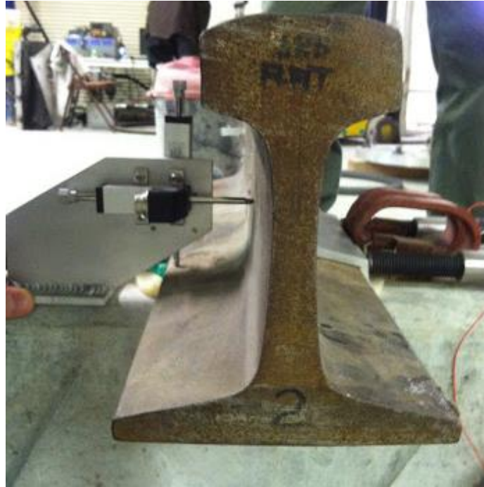
Figure E5: Position of linear potentiometer fixture on the rail (UIUC Lab).
