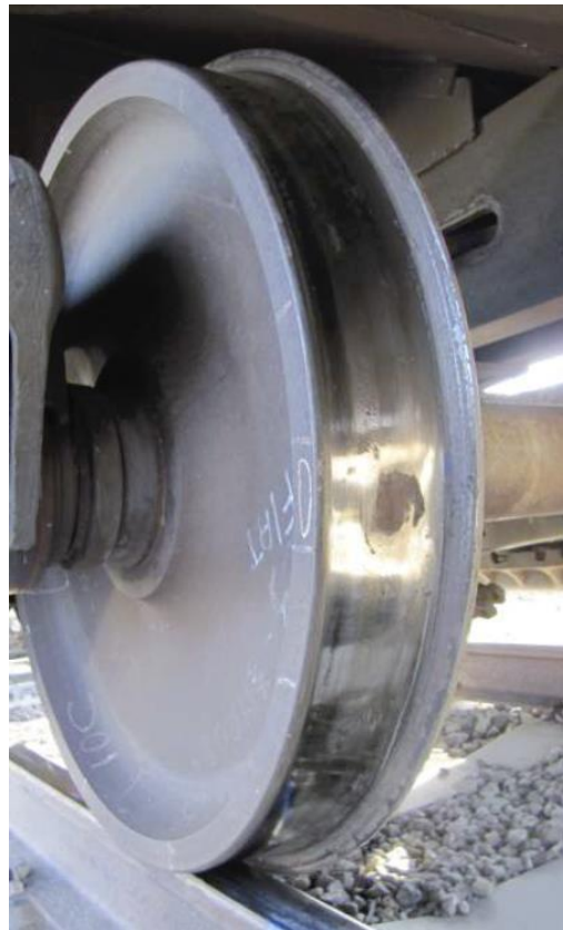
Figure E10: Flat spot on freight car wheel.
