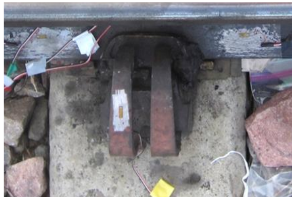
Figure 10: Location of strain gage on fastening clip.
