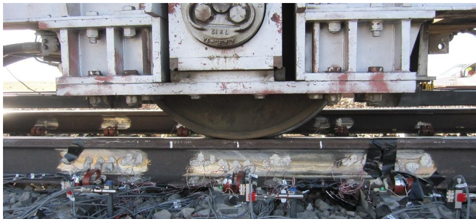
Figure 6: Track Loading Vehicle (TLV) in operation.
