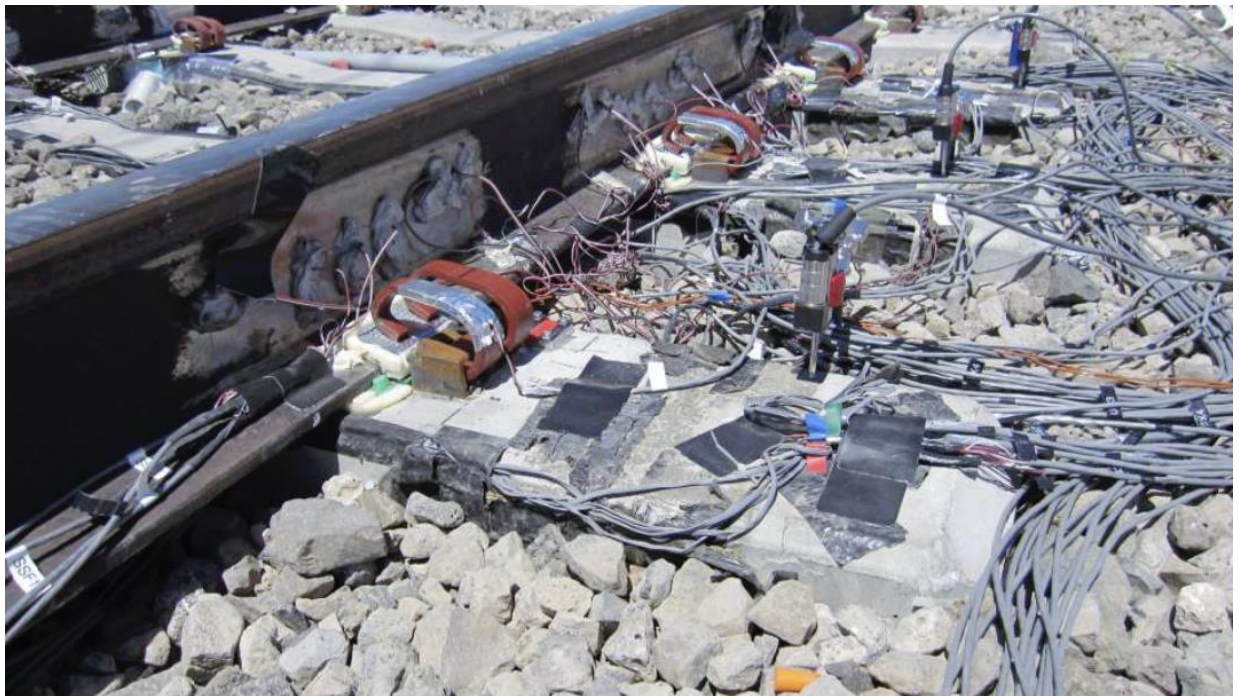
Figure E2: Expanded view of fully instrumented rail seats on tangent track.
