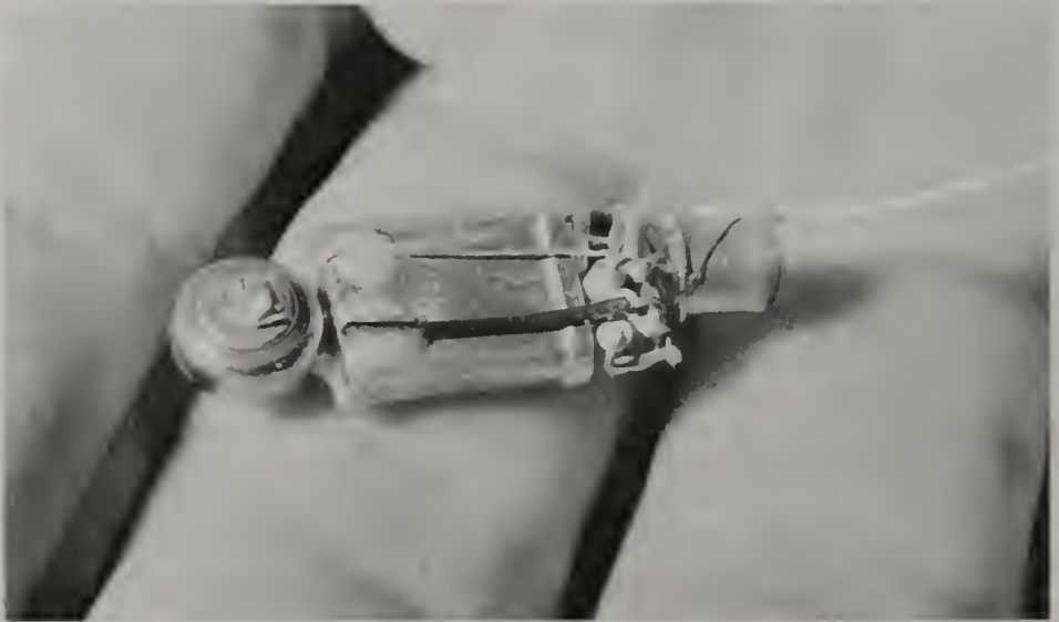
Fig. 1. - (Above) Swainson's thrush carrying a 1.3-g radio transmitter of the type currently in use (Cochran 1980). (Below) a 2.2-g transmitter of the type used in the study reported in this paper.
