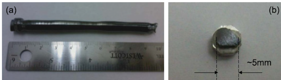
Figure 3.1: Single crystal \text{Mn}_3\text{O}_4 grown by Dr. Min-jung Kim [33]. All samples used in this thesis are diced from this crystal. (a) Crystal as grown. (b) A fractured piece with surface normal to [110] mounted on an aluminum holder.
