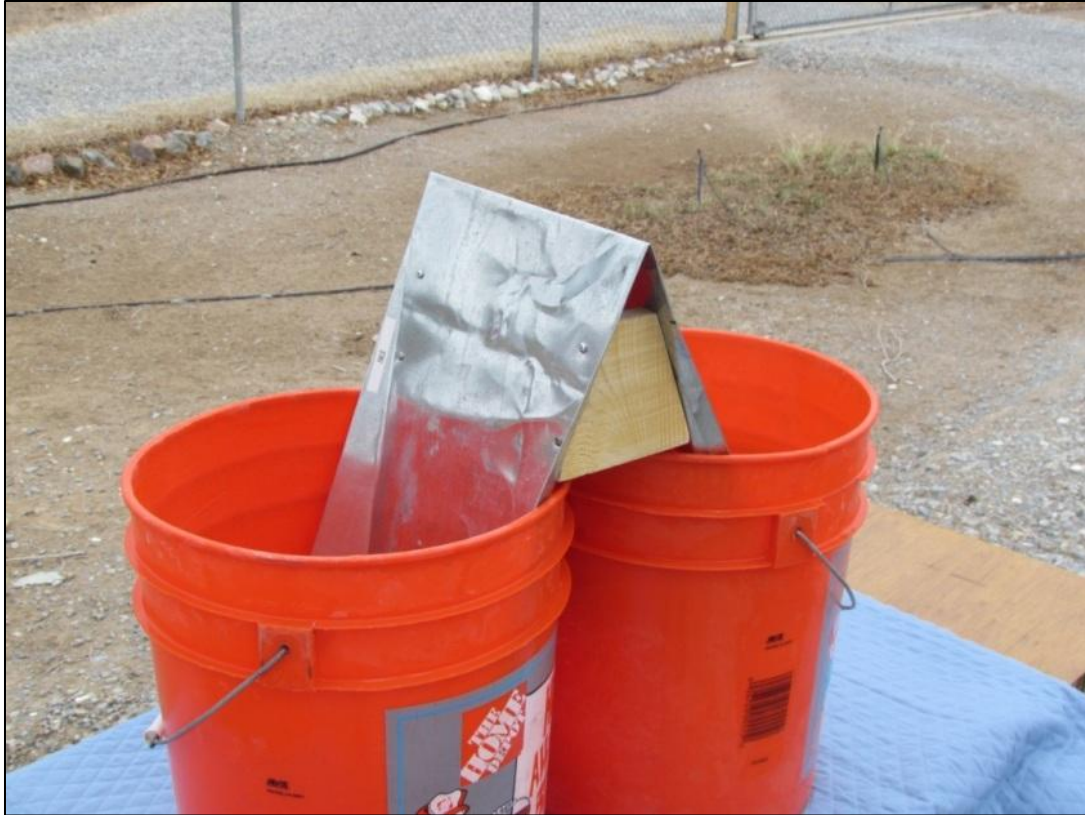
Figure 3: Macroinvertebrate sample splitter used to quarter invertebrate samples taken during the winter and spring sampling periods. (Photo: Hal Fairfield)
