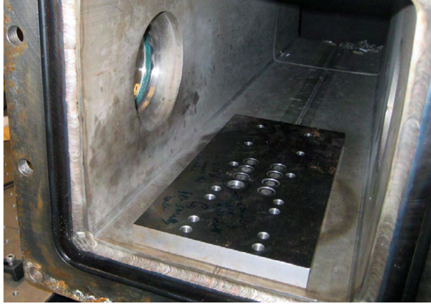
Figure 2.4: An image of the base plate mounted in the test section. The front flange is off, and the view is facing downstream in the facility
