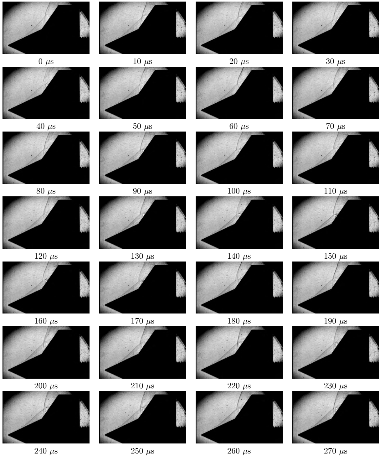
Figure E.7: High speed imaging for the M7.2 nitrogen flow field is shown. The interframe time is 10\mu s and exposure time is 1\mu s . Flow is from left to right.
