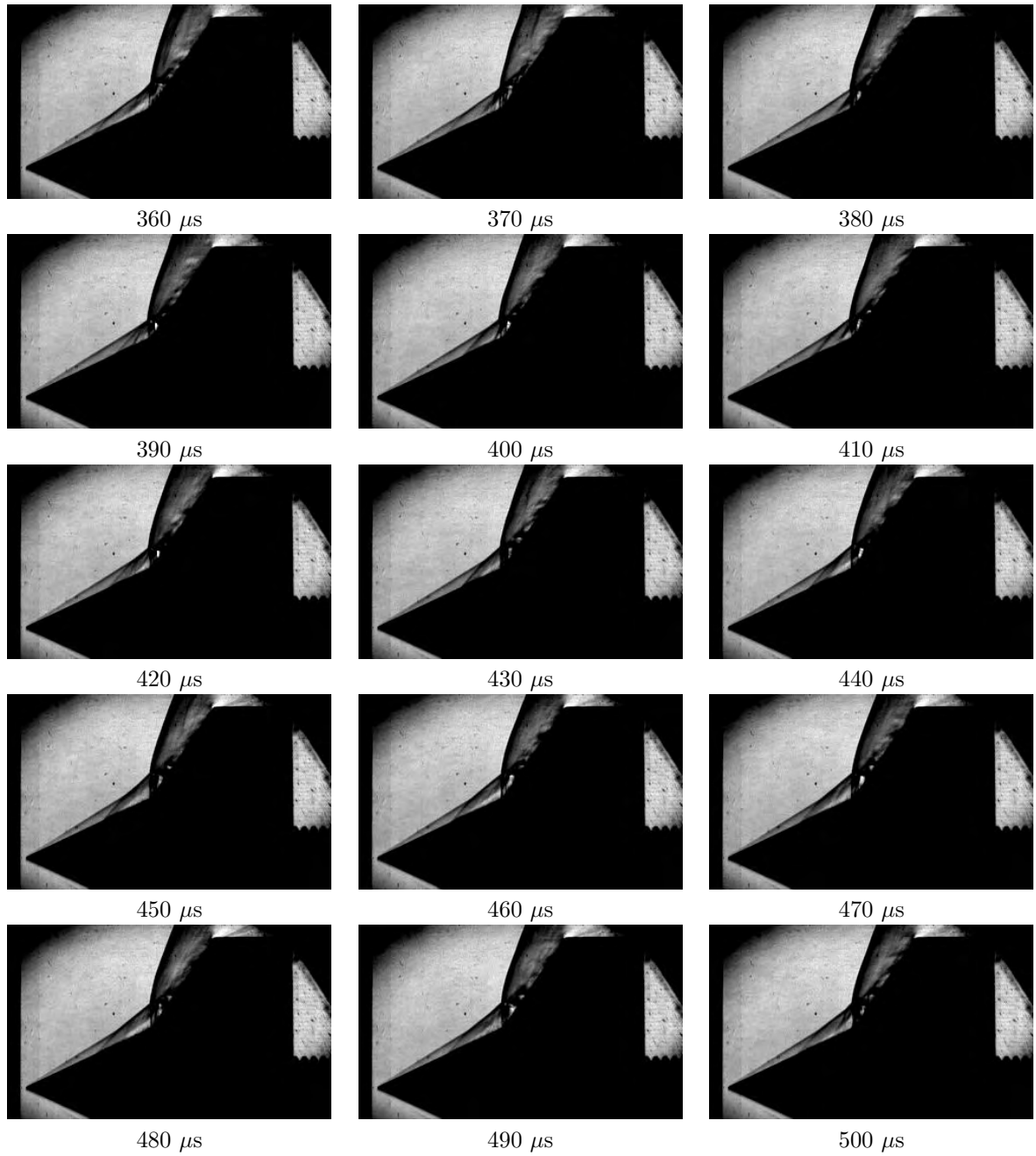
Figure 5.14: Movement in various parts of the flow field is shown for the M4.3.6 test condition in air. The interframe time is 10 \mu s , and the exposure time is 1 \mu s . Flow is from left to right.
