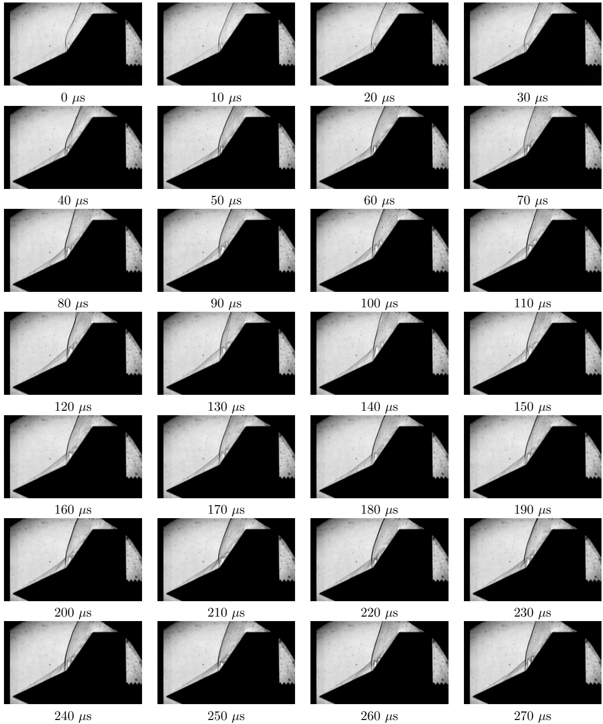
Figure E.8: The first half of the high speed imaging for the M4_3 nitrogen flow field on the double wedge is shown. The interframe time is 10\mu s and exposure time is 1\mu s . Flow is from left to right.
