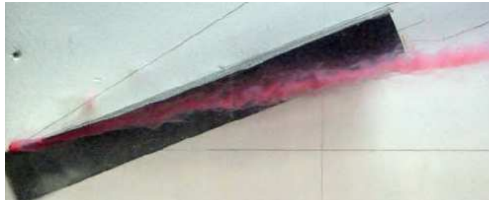
Figure 2.3 Ink visualization for a single winglet on a flat plate.
