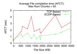
Fig. 16. Average file completion time (AFCT) with 1 YouTube server (small files)
