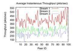
Fig. 11. Avg Instantaneous Throughput Per Peer for Streams 1, 2 and 3
