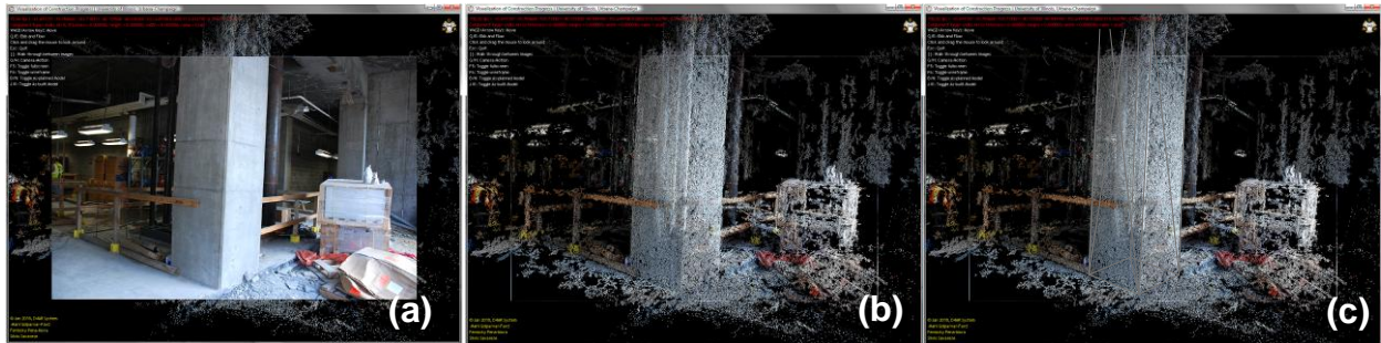
Figure 5.14. (a) Rendered photo of the column automatically registered with the point cloud; (b) point cloud from the same viewpoint without the image; (c) reconstructed shape.
