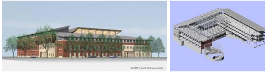
Figure 14. Snapshots of the IFC-based 3D model generated for the Residence Hall Project. Drawings used to generate the 3D model courtesy of the University of Illinois, Urbana-Champaign's Facilities and Services; Used by permission.
