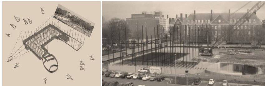
Figure 1.5. Camera Location of randomly taken photographs after the SfM algorithm; (b) Augmented photograph representing the as-planned model superimposed on a photo (Photo Subject: College of Business Inst. Facility, UIUC).
