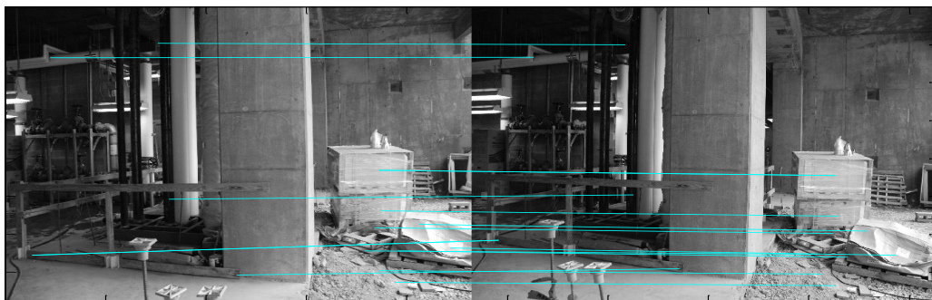
Figure 5.3. A total of 849 SIFT features were matched in this image pair. For visibility, only 14 of these matched features are shown.
