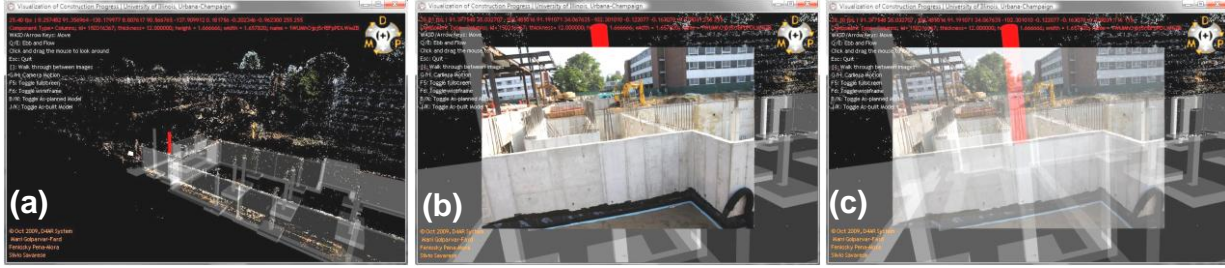
Figure 4.13. (a) The concrete circular column is manually colored with red as behind-schedule; (b) the column seen from a camera viewpoint while image is fully opaque; (c) same viewpoint as that of (b) while image is semi-transparently rendered allowing a see-through on the element.
