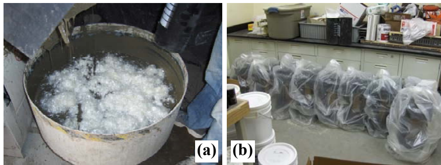
Figure 3.23. (a) Preparation of ECC mixture, and (b) curing of specimens after casting
