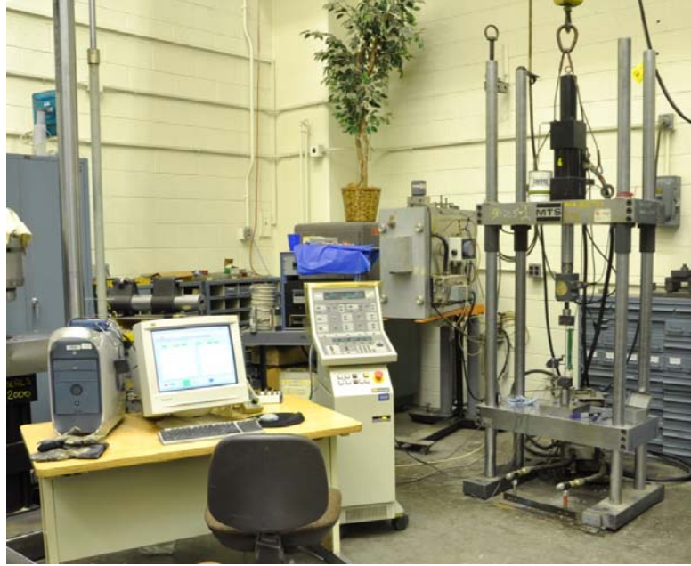
Figure 3.12. Uniaxial testing of threaded rods using servo-hydraulic loading frame
