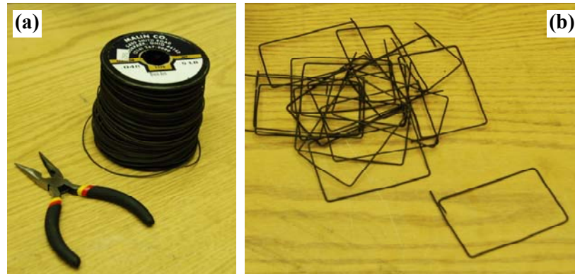
Figure 3.14. (a) Smooth black annealed wire in continuous rolls and (b) rectangular stirrups prepared as transverse reinforcement for small-scale columns
