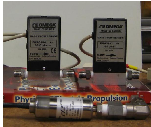
Figure 3.6: Flow sensors. Top Left: Omega Engineering FMA3104 series MFM. Top Right: Omega Engineering FMA3107 series MFM. Center Bottom: Cole-Parmer 68072-52 Type Pressure Transducer.
