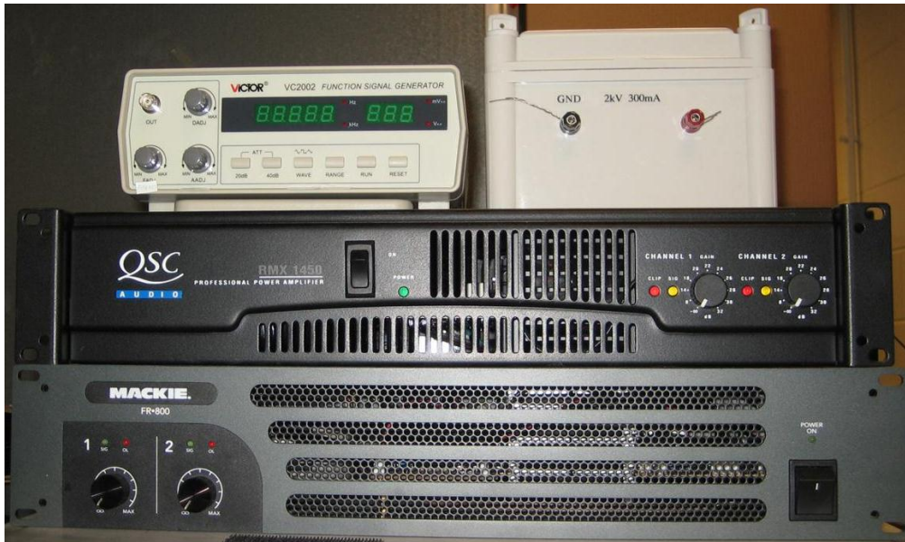
Figure 3.3: MCD Thruster power supply. Top left: Victor VC2002 Function Generator. Top Right: Custom 100:1 Solid Core Transformer. Center: QSC Audio RMX 1450 1400 W 2 Channel Amplifier. Center Low: Mackie FR800 800 W 2 Channel Amplifier
