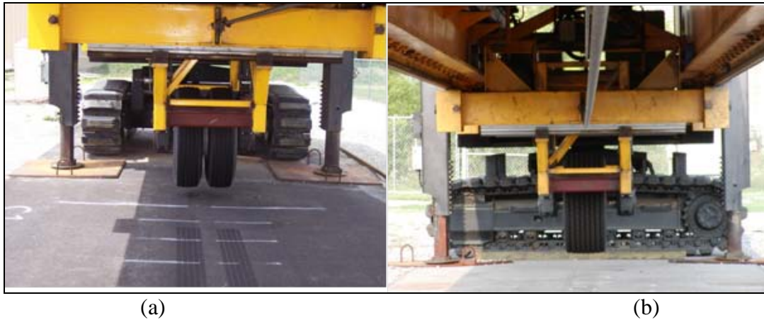
Figure 4.10 Advanced Transportation Loading ASsembly (ATLAS) with a (a) dual-tire assembly; and (b) wide-base tire
