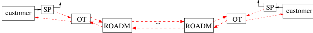
Figure 2.4: Illustration of optical B&R operation steps. A 50/50 optical passive splitter (SP) is preinstalled at the customer's transmission side.
