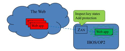
Figure 5.1: Deployment of ZAN. ZAN works by interposing on key states and events of web apps within the browser to detect candidates for adding protection automatically.
