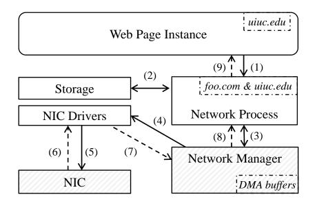
Figure 3.2: IBOS work flow. This figure enlarges the right half of Figure 3.1 and shows how our IBOS subsystems interact when a web page instance from uiuc.edu issues a network request to foo.com. Subsystems are shown in boxes and solid and dotted arrows represent IBOS messages for outgoing and incoming data respectively. The reference monitor (which is not shown here) checks all these messages to enforce security properties.
