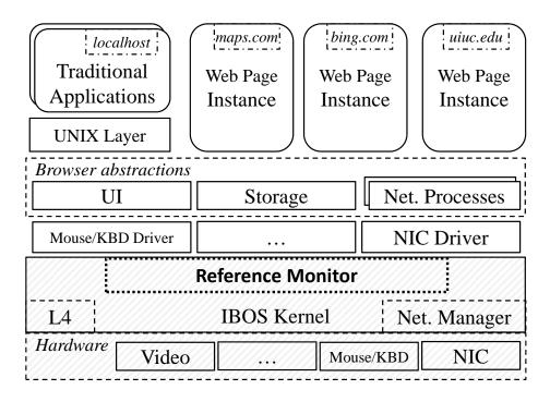
Figure 3.1: Overall IBOS architecture. Our system contains user-mode drivers, browsers API managers, web page instances, and traditional processes. To manage the interactions between these components, we use a reference monitor that runs within our IBOS kernel. Shaded regions make up the TCB.
