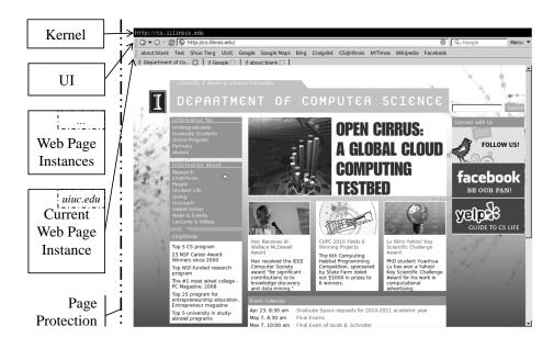
Figure 3.3: IBOS display isolation. This figure shows how IBOS divides the display into three main parts: a bar at the top for the kernel, a bar for browser chrome, and the rest for displaying web page content. The IBOS kernel enforces this isolation using page protections and *without* relying on a window manager.
