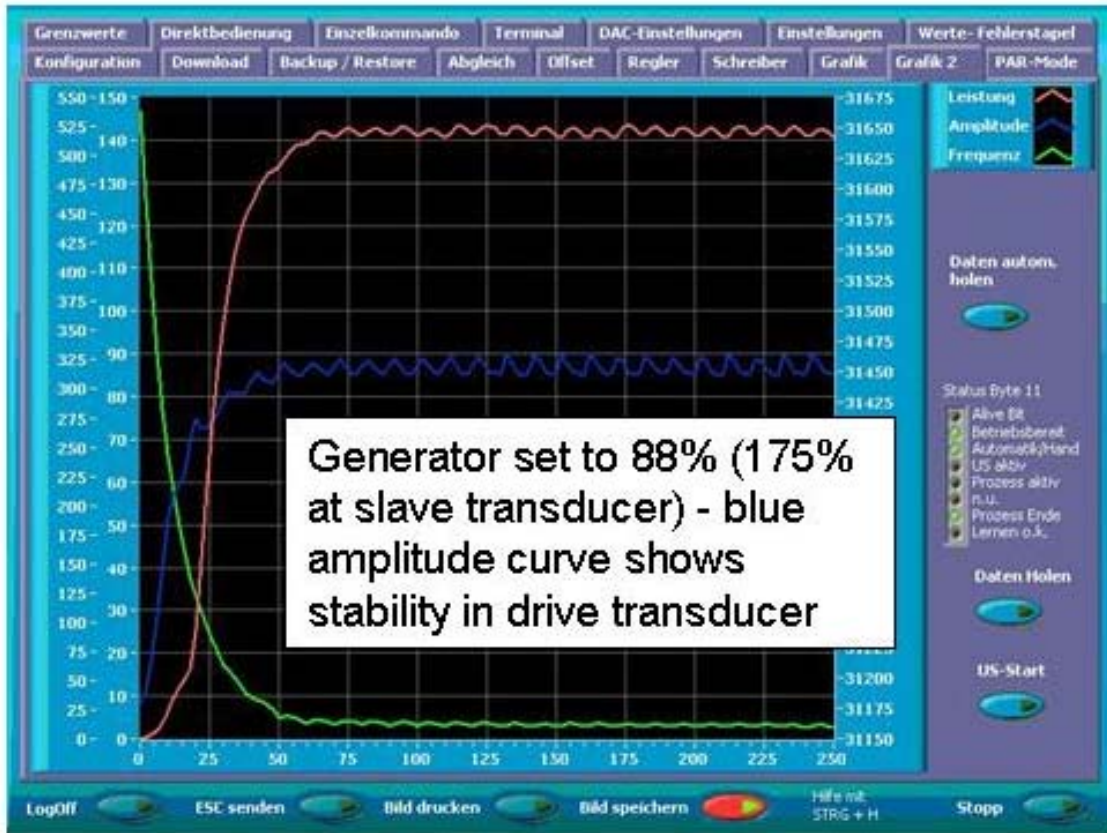
Figure 4.9 – DIASIM graphs before and after entering destabilized zone
