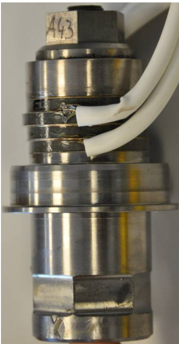
Figure 1.8 – Transducer failure due to shifting crystals
