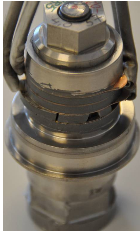
Figure 1.7 – Transducer failure due to cracked crystals
