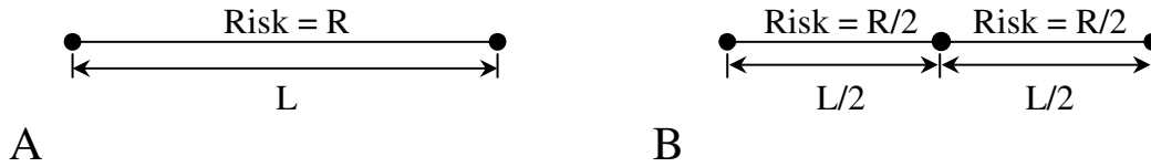
Figure 5.14: Illustration of a Track Segment (A) Without Division and (B) With Equal Divisions
