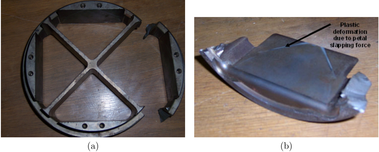
Figure 2.6: a) Back-view picture of the knife blades showing the nature of the fracture and the broken quarter piece. b) A close up of the broken quarter piece indicating the plastic deformation caused by the petal slapping force.
