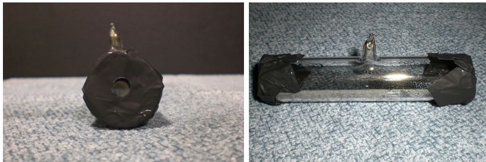
Figure 4.2: (Left) End-on and (right) side-on images of a 10 cm long gas cell with black foil end caps introduced to mitigate uncollimated light from contributing to the output signal.
