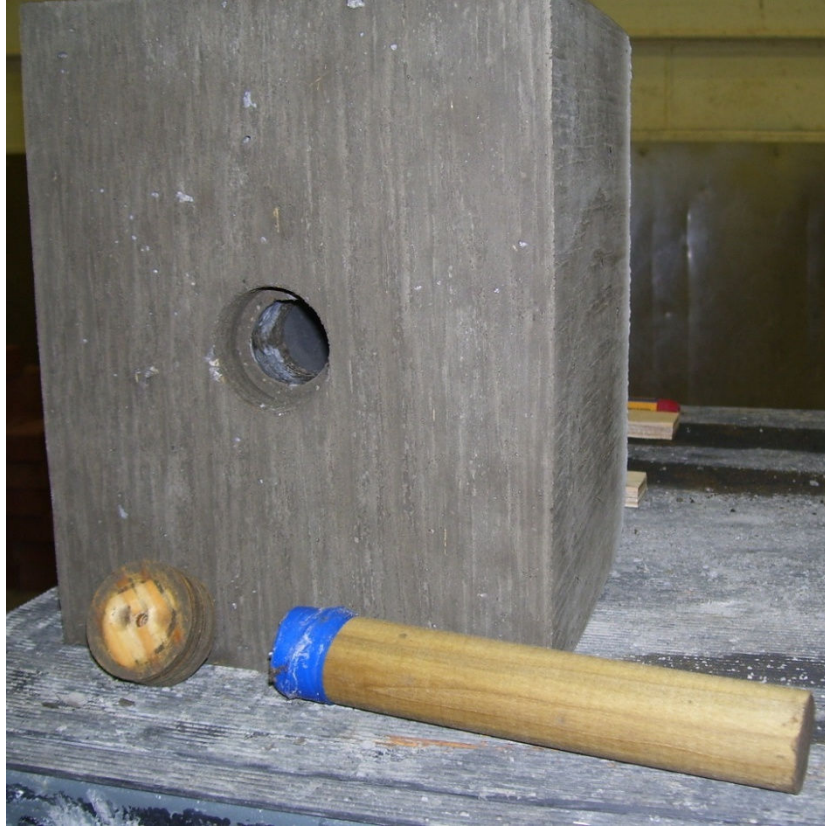
Figure D.5 Wooden dowel and cylindrical piece removed during demolding
