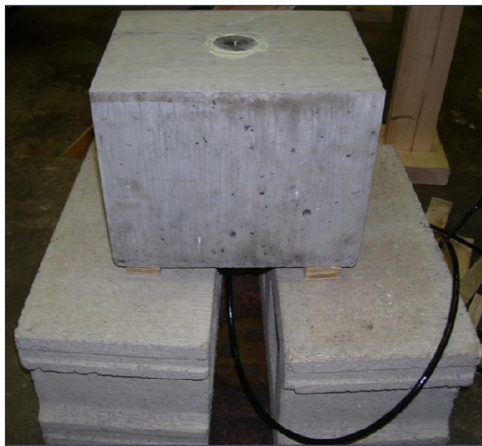
Figure 6.2 Concrete block prepared with pressure transducer
