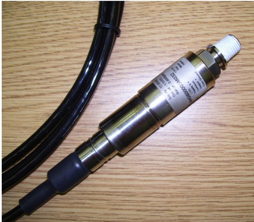
Figure 5.2 Submersible pressure transducer used in the load tests
